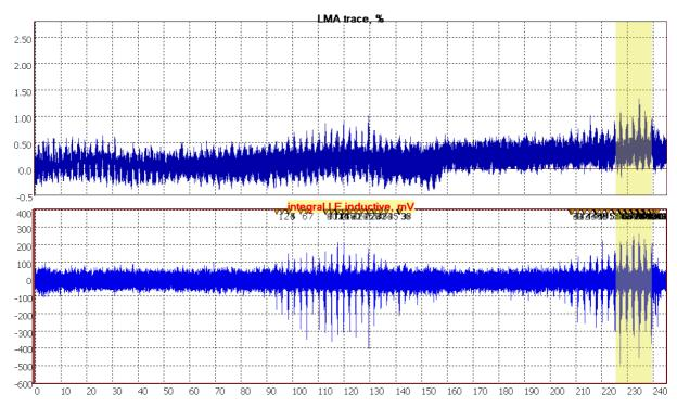
Figure 5. LMA and LF traces for the rope running 5400 t-km.
