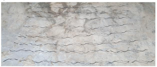
Figure 6. Broken wires of one strand after its unstranding.
