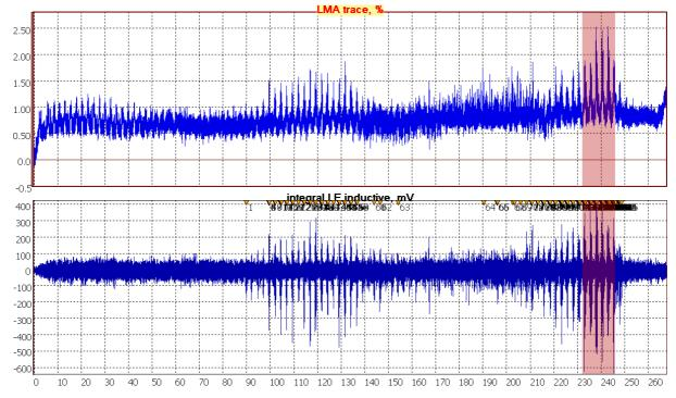
Figure 5. LMA and LF traces for the rope running 5900 t-km.
