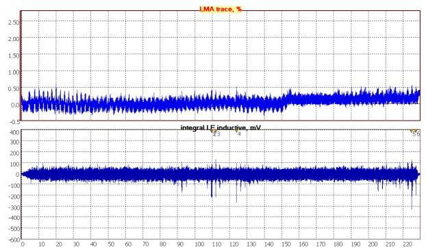
Figure 3. LMA and LF traces for the rope running 4545 t-km.
